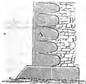
Fig 7—Represents a section of a wall in which the face is of cut stone, with the tails of the blocks thinned off, and the backing of rubble A, section of face block. B, rubble backing.
